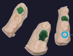
Rapid printing, the exposure time on a 4K mono printer is only 2.5s per layer, 110 crowns are printed within 40mins, and 7 partial denture frames are printed within 2.5 hours.
